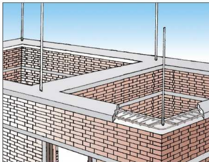
Figure 63 Reinforced concrete band
